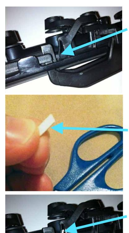
Identify the spring that holds key pad 24 closed at rest.
