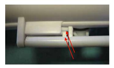
To return the long key to its correct position, simply reverse the above procedure paying particular attention to the springs which must be positioned as shown for the key to function correctly.
