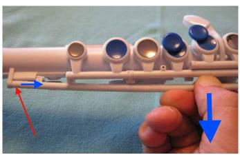
Now pull more firmly towards you so that the left hand end of the rod comes out of it's seating, marked by the red arrow. The long key will be released from the left hand end and can now be removed from the instrument.
