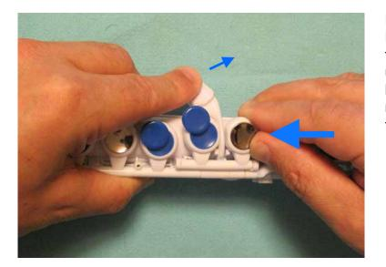
Hold the flute securely as shown. Depress the G# key with the left index finger. With the right hand, lift the key up and push very firmly to the left. The key will bend so that it can be released from it's axle location hole on the right side. See next image.
