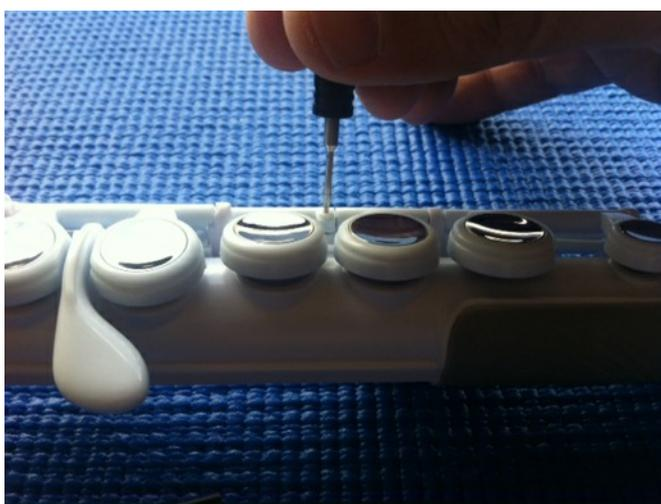
If key B is closing before key C then you should adjust the screw out by turning it counter-clockwise. If key B is closing after key C then you should adjust the screw in by turning it clockwise. This is the principle for adjusting all the keys. If you are satisfied with the relationship between B and C, move on to step 2.
