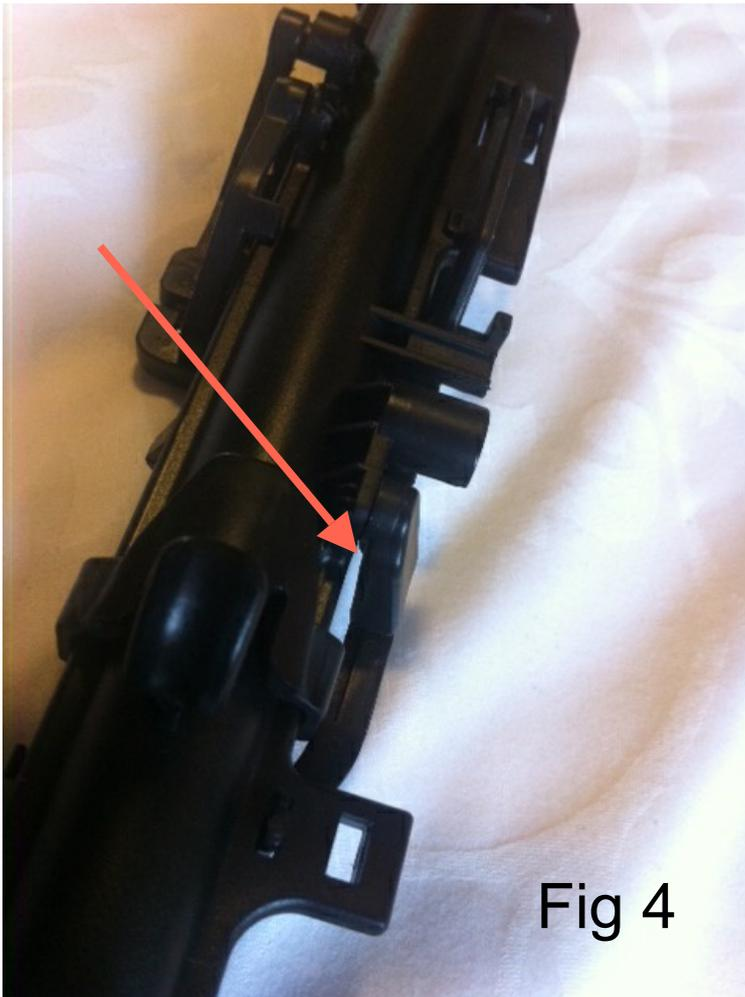
Now looking at the instrument from the back, insert a flat head screwdriver into the slot indicated by the red arrow in Fig 4. Lever the key away from the body while at the same time pulling the key with your other hand. This will release the pivot clip from the body.
